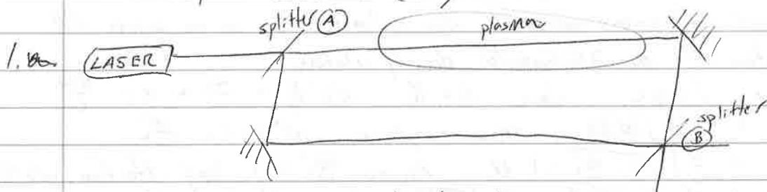
A single beam is split into two at point (A). Due to different index of refraction in the plasma vs air, the reference and plasma beam will have different phase when meeting at point B. In the plasma,  $\omega^2 = \omega_p^2 + k^2 c^2 \rightarrow N^2 = 1 - \frac{\omega_p^2}{\omega^2}$  so  $N$  (ne), hence a measurement of the electron density can be made.
