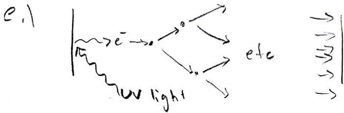
the first current "bump" occurs when the original electrons reach the anode.
