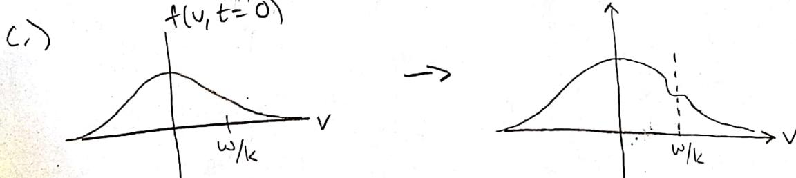
d.) For  $E(x, t \rightarrow \infty)$  to remain finite, the wave must have more energy than the particles take from it.
